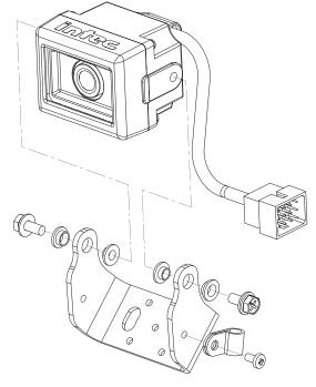
2 Assemble the camera to the bracket then secure the camera pigtail to the bracket with the "P" Clamp provided, as shown below.
